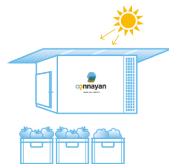
Solar cold rooms of 2 to 5 MT capacity, costing $10,000 – $16,000 per system
